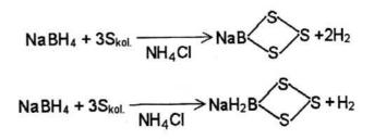
The reduction products in the above reactions are sodium borohydride sulphides that can be quantitatively oxidized to sulphates:
